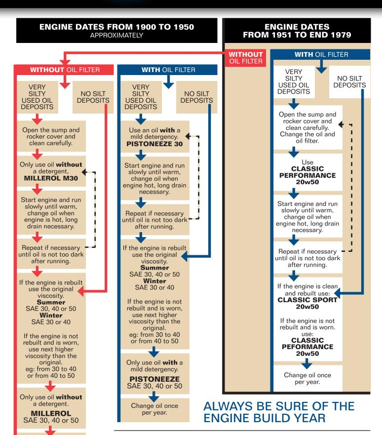
The best time to change the oil is at the end of the driving season. Change the oil and run the engine until hot. Store the car. During storage never start and stop the engine without the oil reaching its normal operating temperature. Don't forget to change the gear and rear axle oils every 4-6 years. Change the brake fluid every year. Grease all necessary parts every year.
